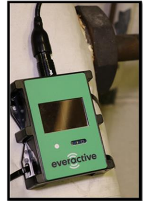
Eversensor (above) connects to harvesting source TEG harness (below) for power and remote temperature measurements.
