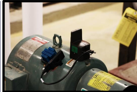
Aerial view of TEG harvester attachment
